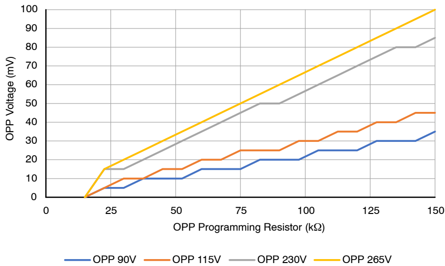
Figure 28. OPP Voltage vs. R_{OPP} for Different Input Voltages
