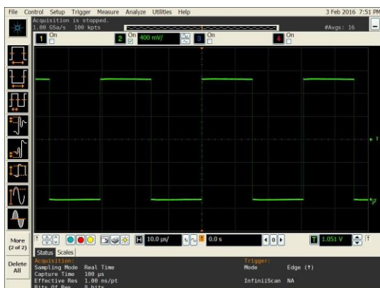
Figure 3. LVC MOS Output Swing ( V_{DD} = 1.8\text{ V} )
