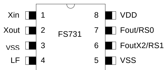
Figure 2. FS731, SOIC Package Pin Assignment
