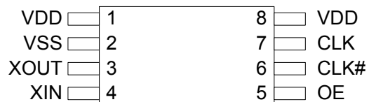
Figure 1. 8-pin TSSOP pinout
