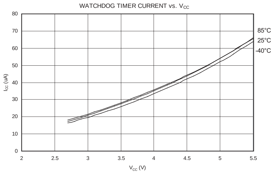
Figure 186. Watchdog Timer Current vs. V_{CC}
