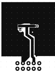
a) 87^\circ\text{C/W} when mounted on a 1\text{in}^2 pad of 2 oz copper.
