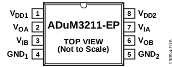
Figure 5. ADuM3211-EP Pin Configuration
