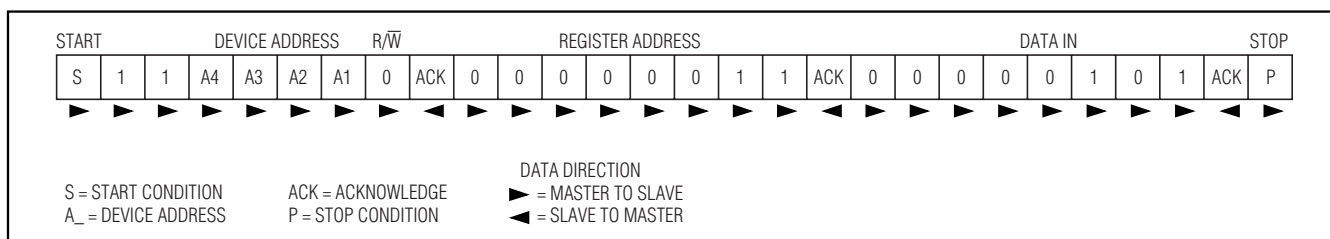
Figure 5. Example—Setting CLK3 to 80MHz
