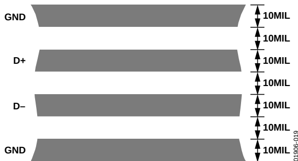
Figure 19. Arrangement of Signal Tracks
